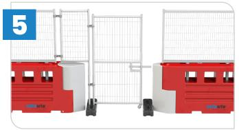
If installing an unframed pedestrian gate, you need to attach an adaption pole to one side of the opening, and a slam post to the other. This is attached to the flag/adaption panel in the same way as the adaption post.
